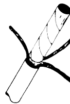
FIGURE 2 GROSS SHIELD PIGTAILS
