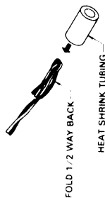
FIGURE 3 TERMINATION OF SPARE CONDUCTORS
