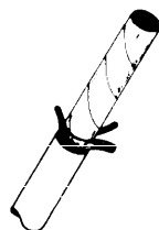
FIGURE 3 TRIMMED PIGTAILS
