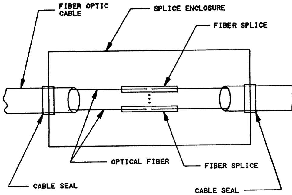
FIGURE 1. Splice assembly.
