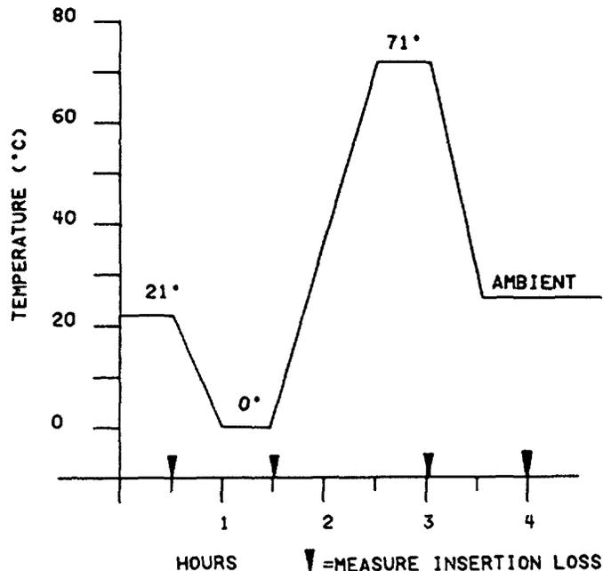
FIGURE 2. Operating temperature range test.
