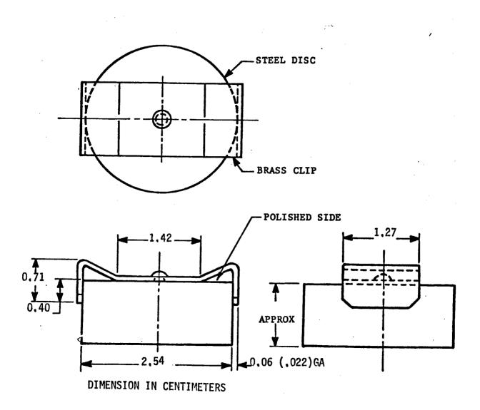
FIGURE 1. Typical test specimens for corrosivity test.
