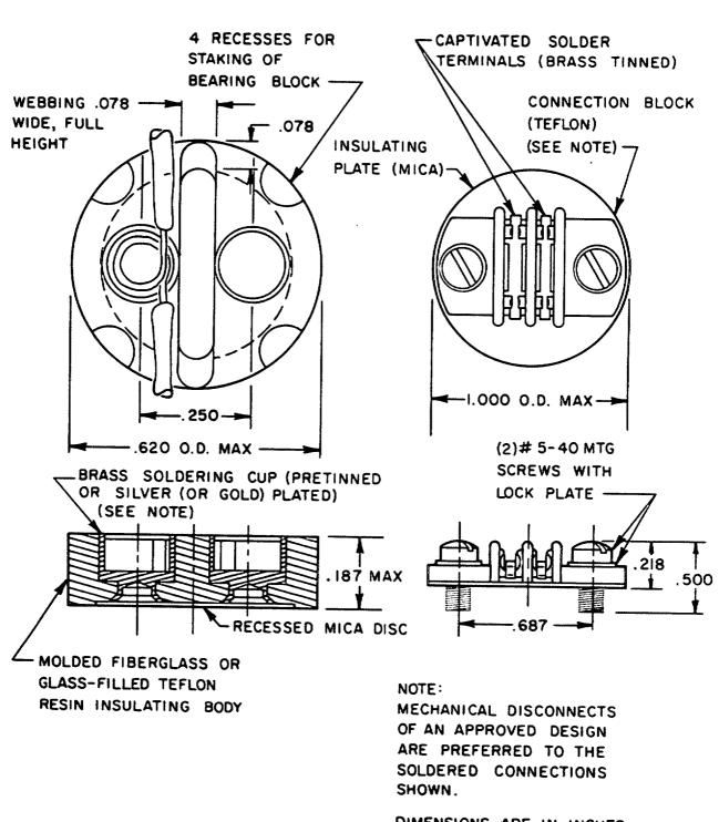
DIMENSIONS ARE IN INCHES AND TOLERANCE IS ±.010 EXCEPT WHERE NOTED.
