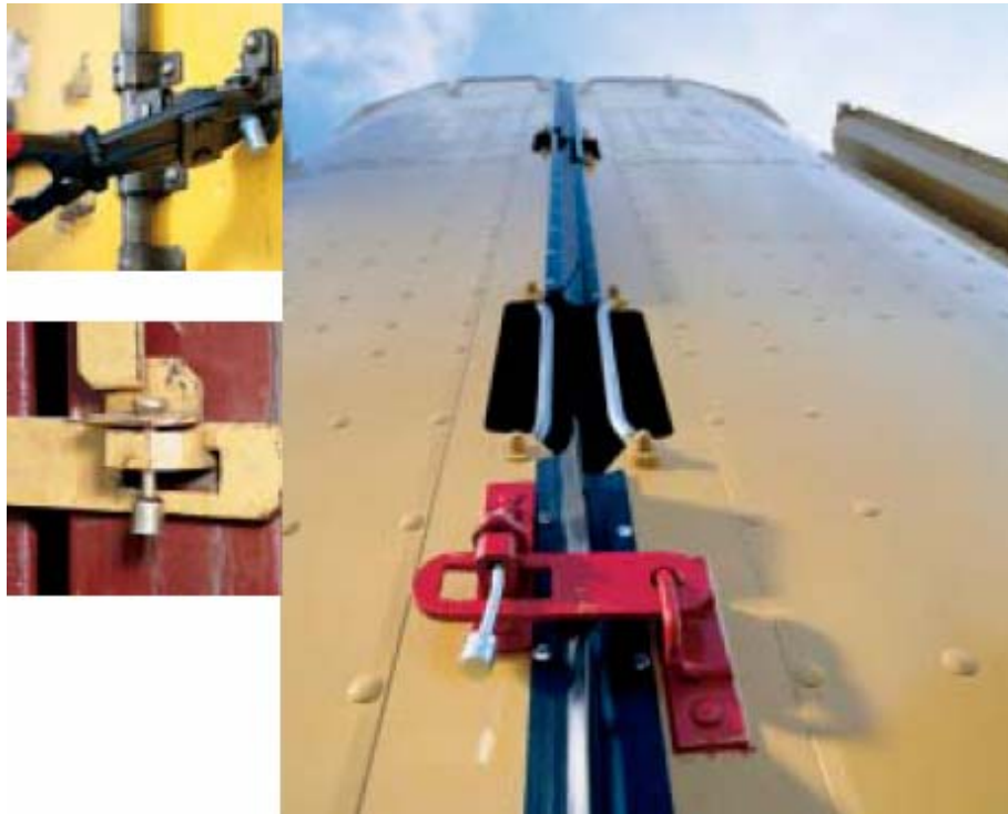
Figure 5-9. Bolt Seal Applications.
