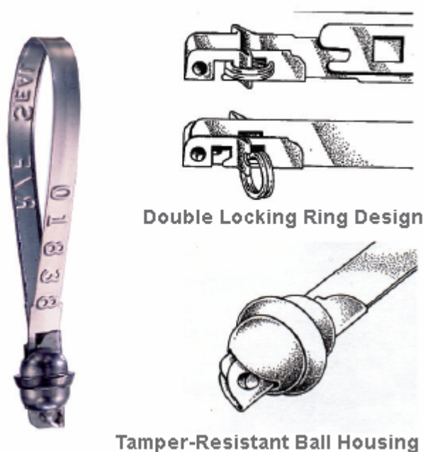
Figure 5-6. Tyden Ball Seal by Tyden Brammel.
