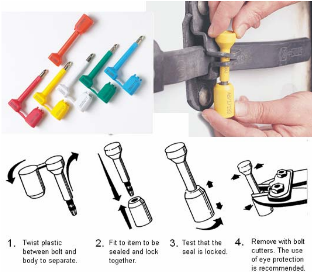
Figure 2-22. Bolt Seal Installation.
