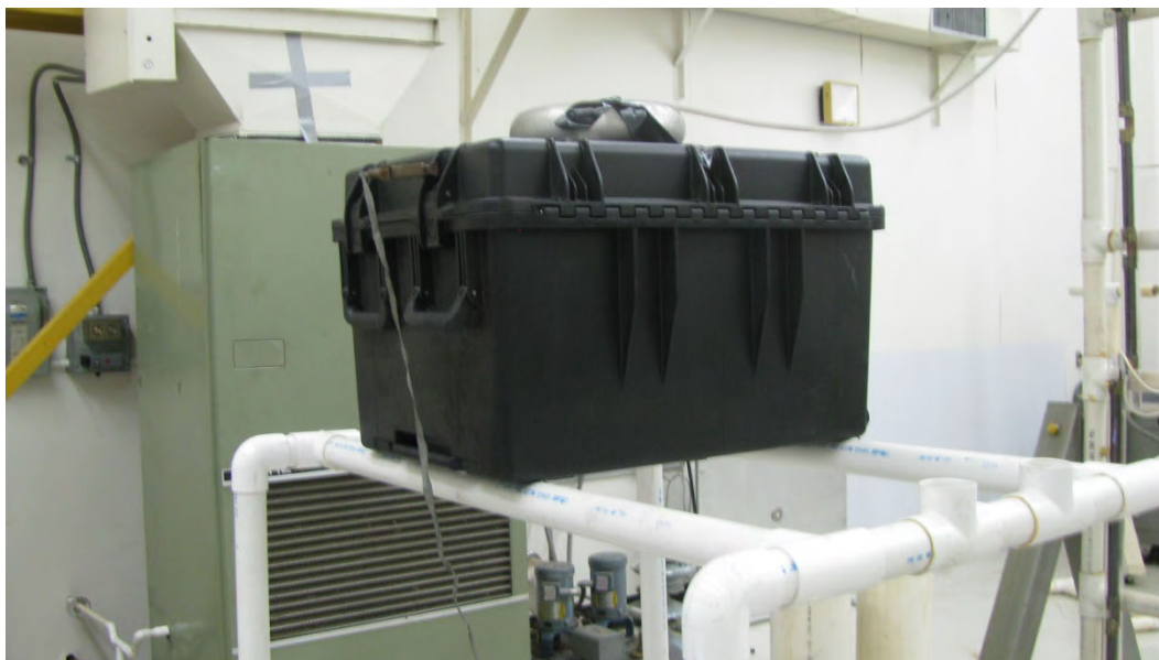
Figure 8: Inert bridgewire inside shipping container Marx test setup
