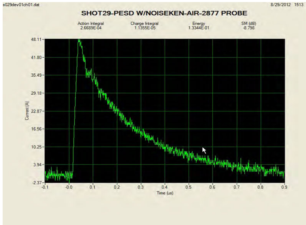
Figure 15: PESD instrumentation test setup output waveform from the Noiseken equipment
