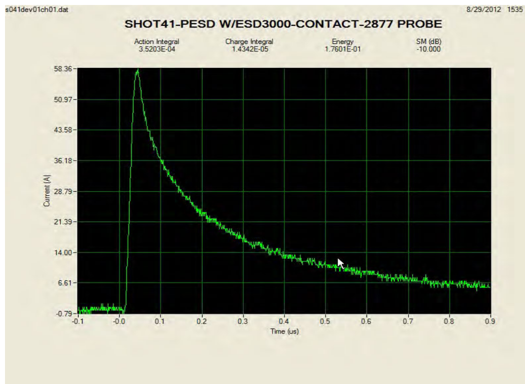
Figure 16: PESD instrumentation test setup output waveform from the ESD 3000 equipment
