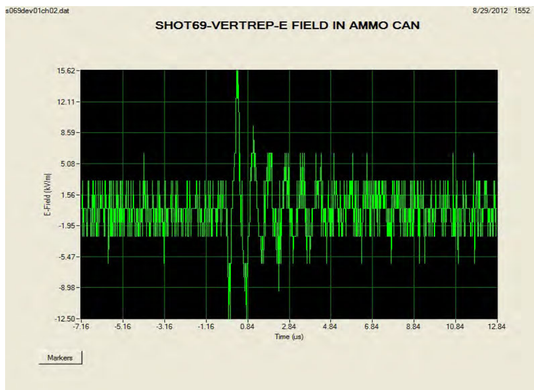
Figure 10: E field probe inside the metal shipping container VERTREP test waveform
