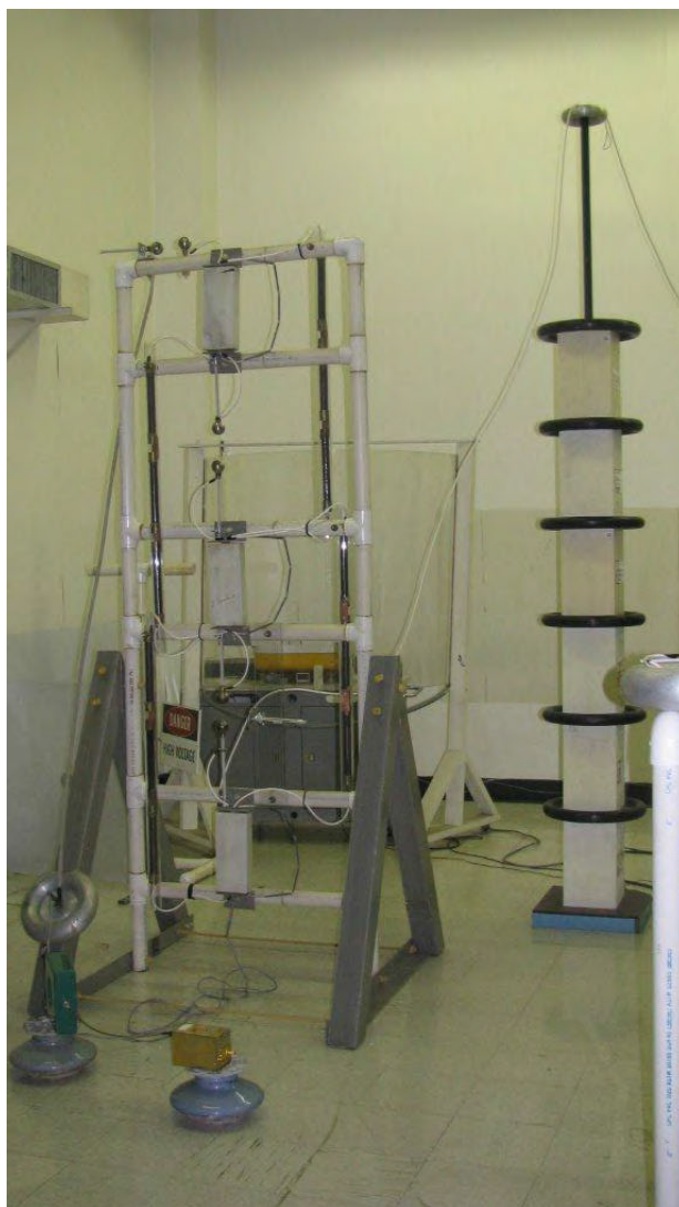
Figure 2: Marx test equipment setup
