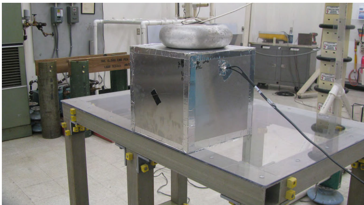
Figure 5: 0.016 inch T-6061 Aluminum test equipment setup
