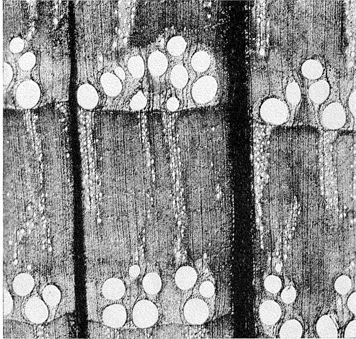
*Figure 2-7. Chestnut oak. Cross section magnified 20 diameters.*
