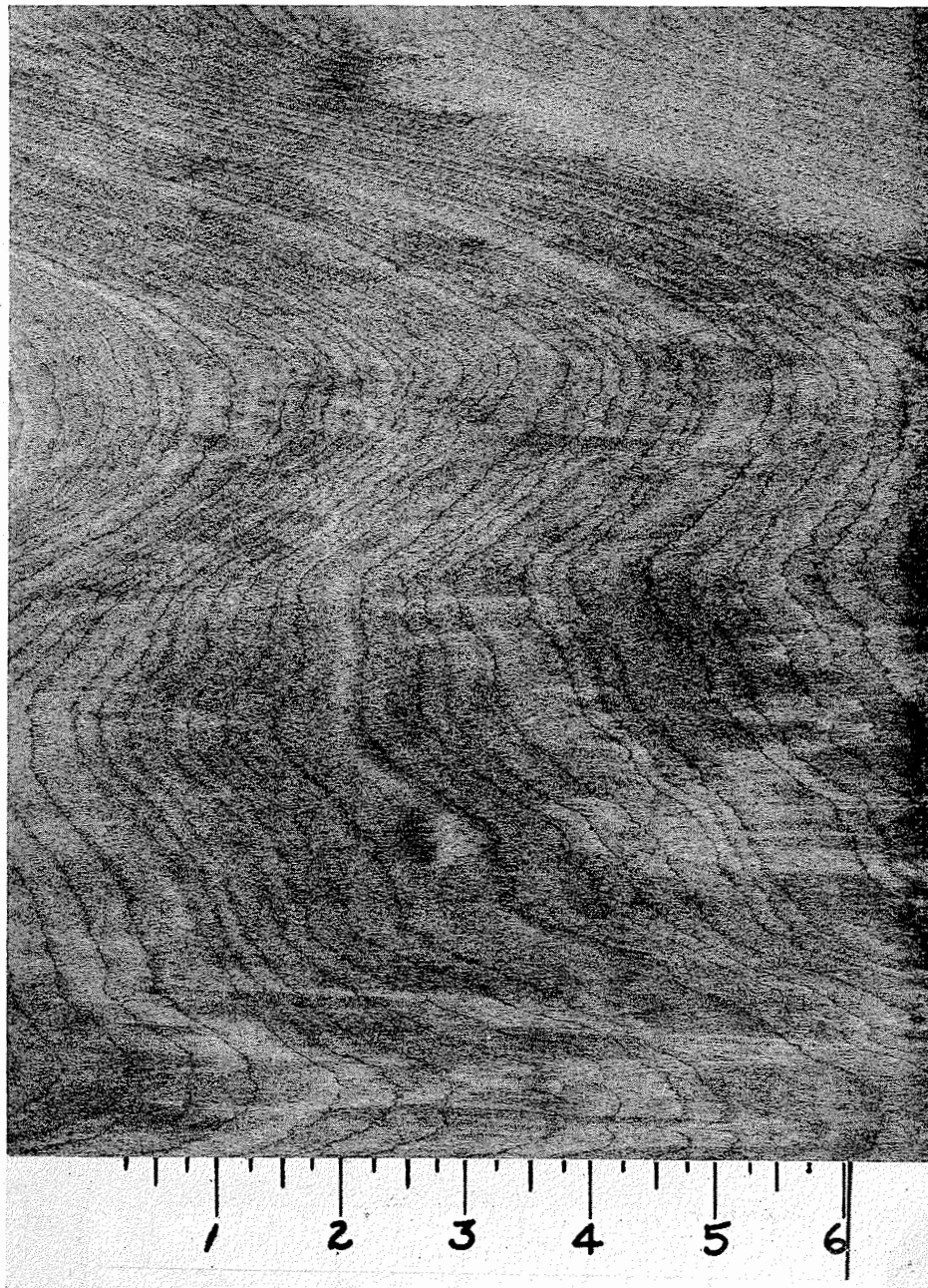
Figure 2-89. Cross grain resulting from butt joint in yellow birch.
