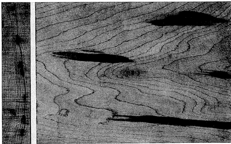
Figure 2-75. Mineral streak.
