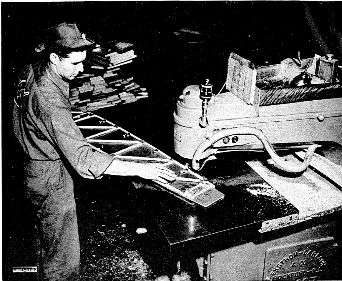
Figure 5-83. Routing wing ribs to contour.
