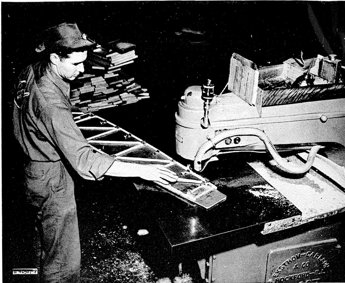
Figure 5-83. Routing wing ribs to contour.
