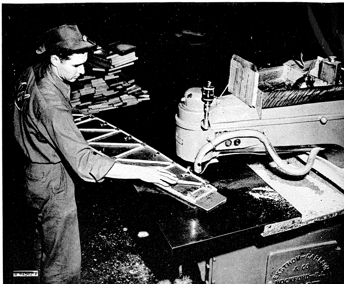
Figure 5-83. Routing wing ribs to contour.
