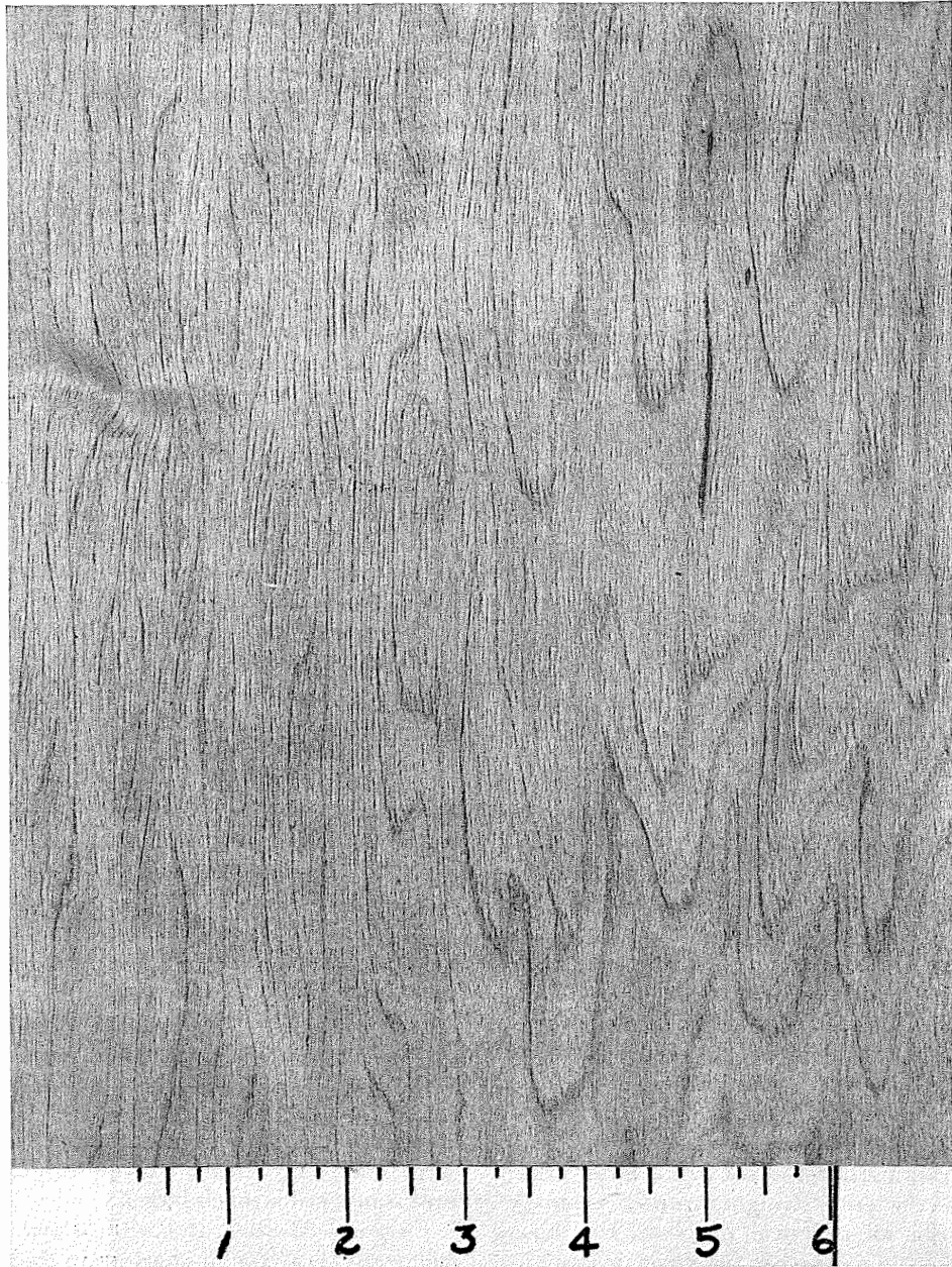
Figure 2-88. Objectionable rough cutting in maple.
