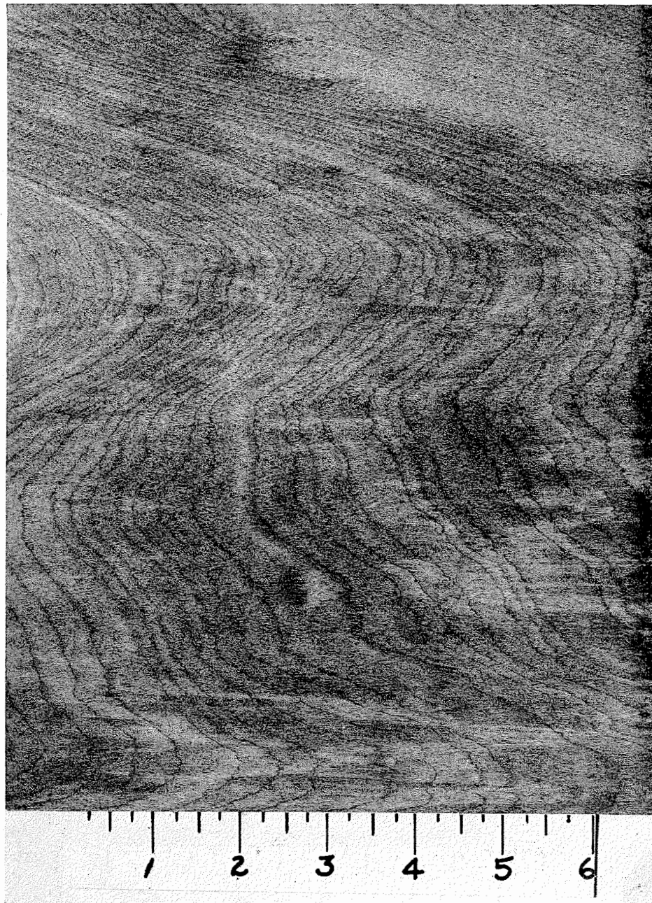
Figure 2-89. Cross grain resulting from butt swell in yellow birch.
