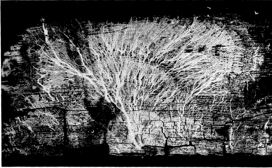
Figure 2-98. Mycelium on oak and the characteristic cracking of typical brown rot.
