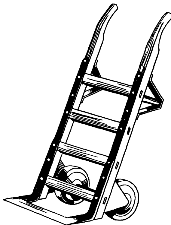
Figure 4-1. Handtruck, warehouse, double-handle type, 2-wheel, solid-rubber tires
