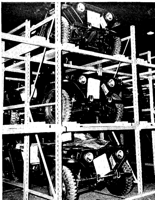
Figure 5-18 Roll-through racks for stacking vehicles in storage
