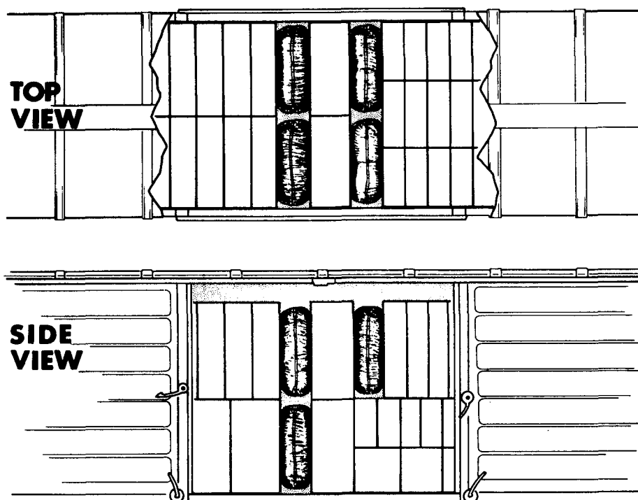
Figure 3-48 Pneumatic dunnage units in various void arrangements
