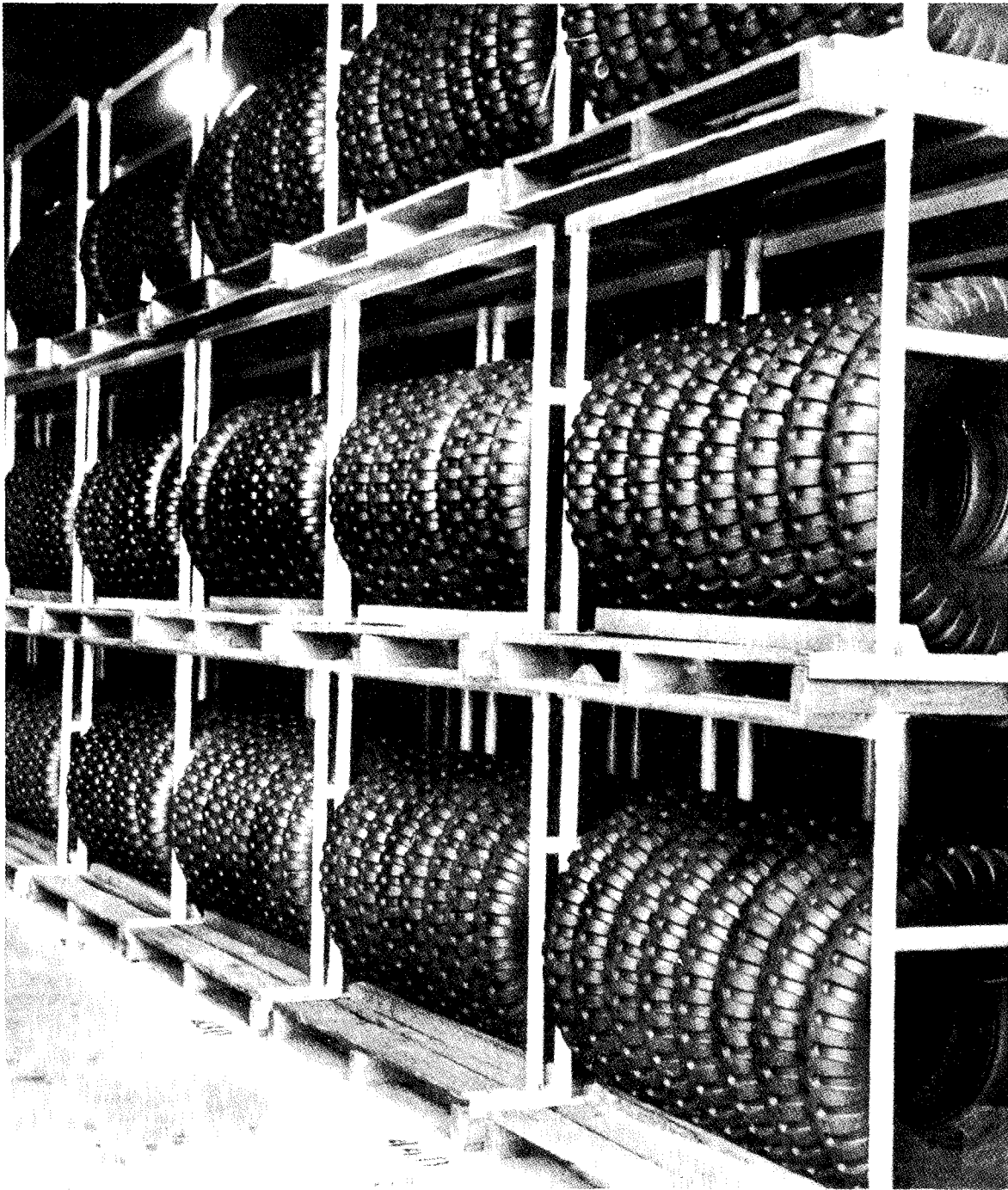
Figure 5-43 Typical storage in pallet support sets
