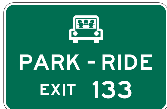
Figure 2E-25. Supplemental Guide Sign for a Park – Ride Facility
