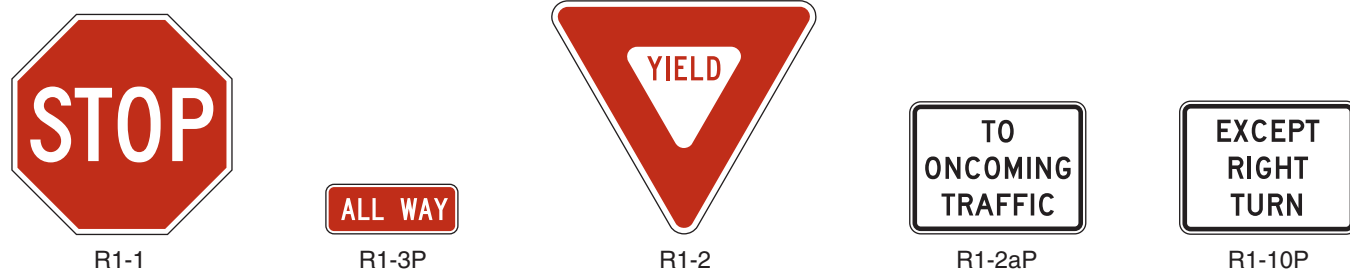
Figure 2B-1. STOP and YIELD Signs and Plaques
