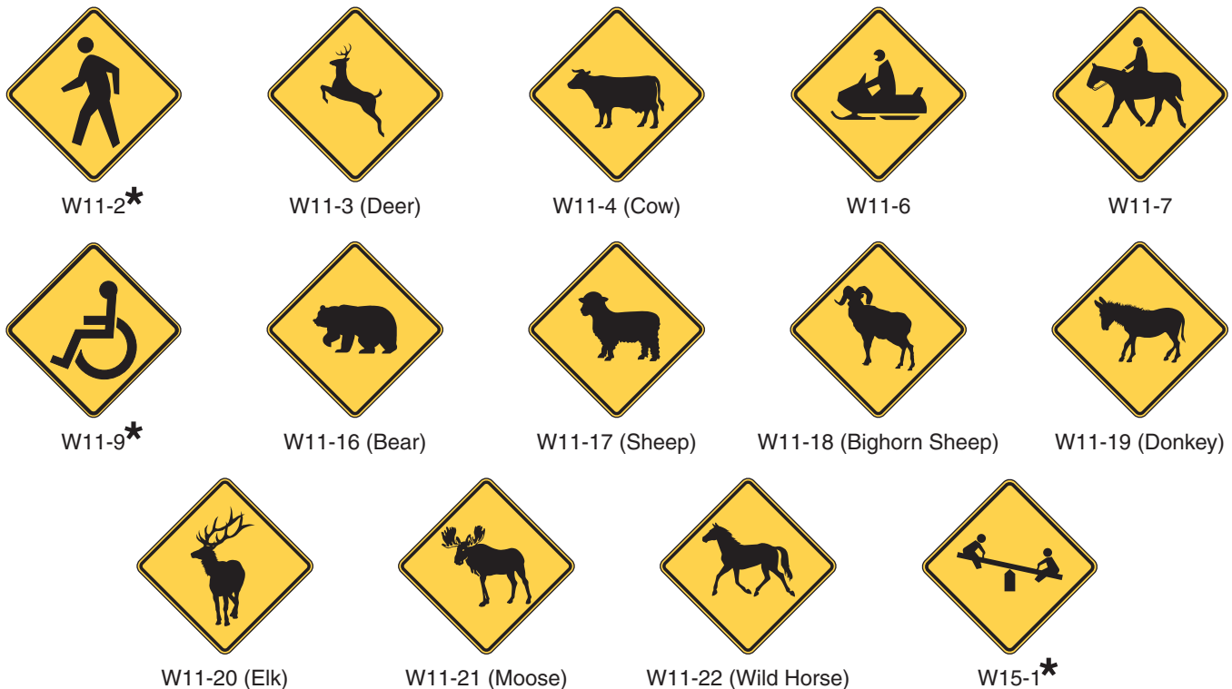
Figure 2C-11. Non-Vehicular Warning Signs
