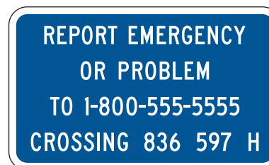
Figure 8B-5. Example of an Emergency Notification Sign
