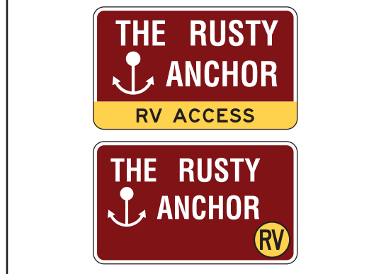
Figure 2J-4. Examples of RV Access Supplemental Messages on Logo Sign Panels
