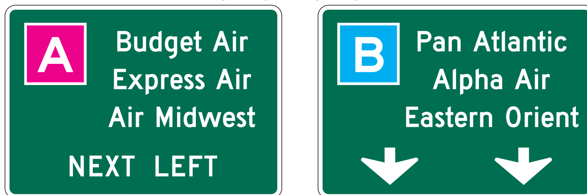
Figure 2D-1. Examples of Color-Coded Destination Guide Signs
