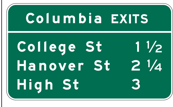
Figure 2E-32. Community Interchanges Identification Sign
