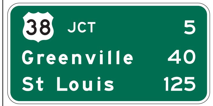
Figure 2E-29. Post-Interchange Distance Sign
