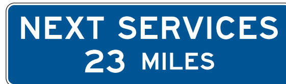
Figure 2I-2. Example of Next Services Plaque
