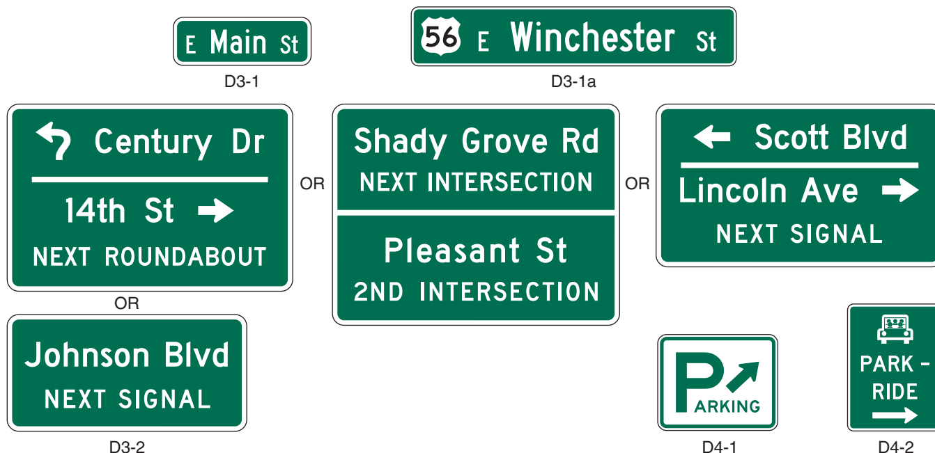
Figure 2D-10. Street Name and Parking Signs
