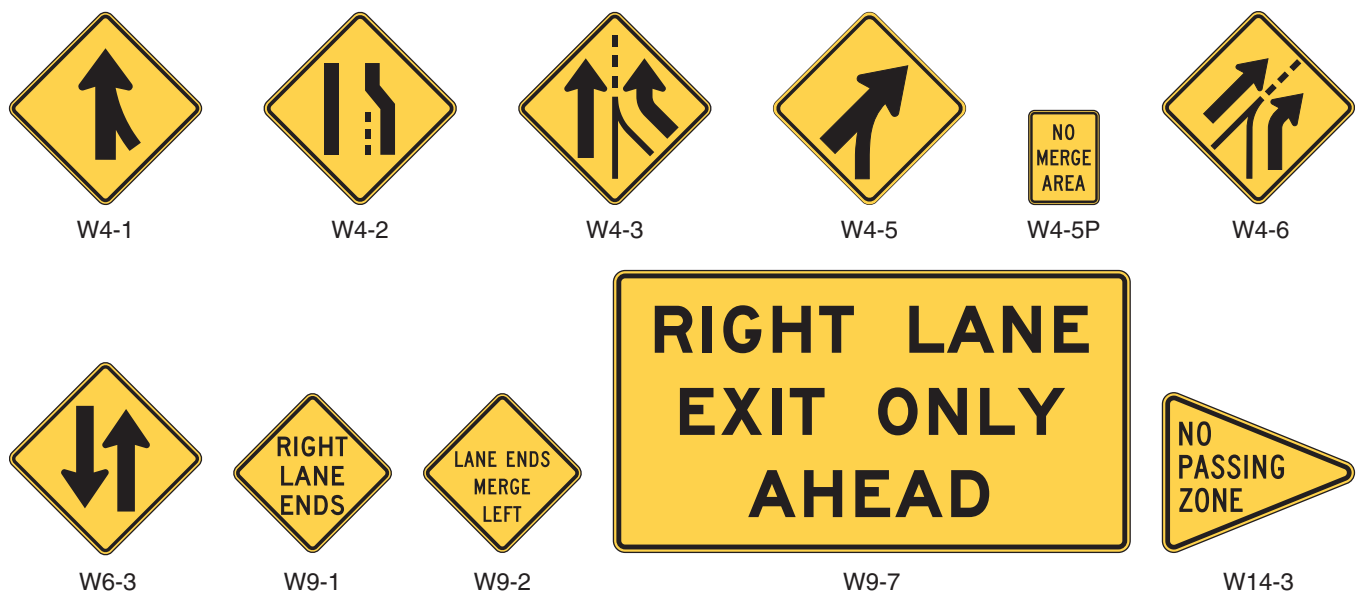
Figure 2C-8. Merging and Passing Signs and Plaques
