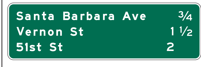
Figure 2E-31. Interchange Sequence Sign
