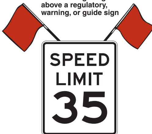
Figure 2A-1. Examples of Enhanced Conspicuity for Signs
