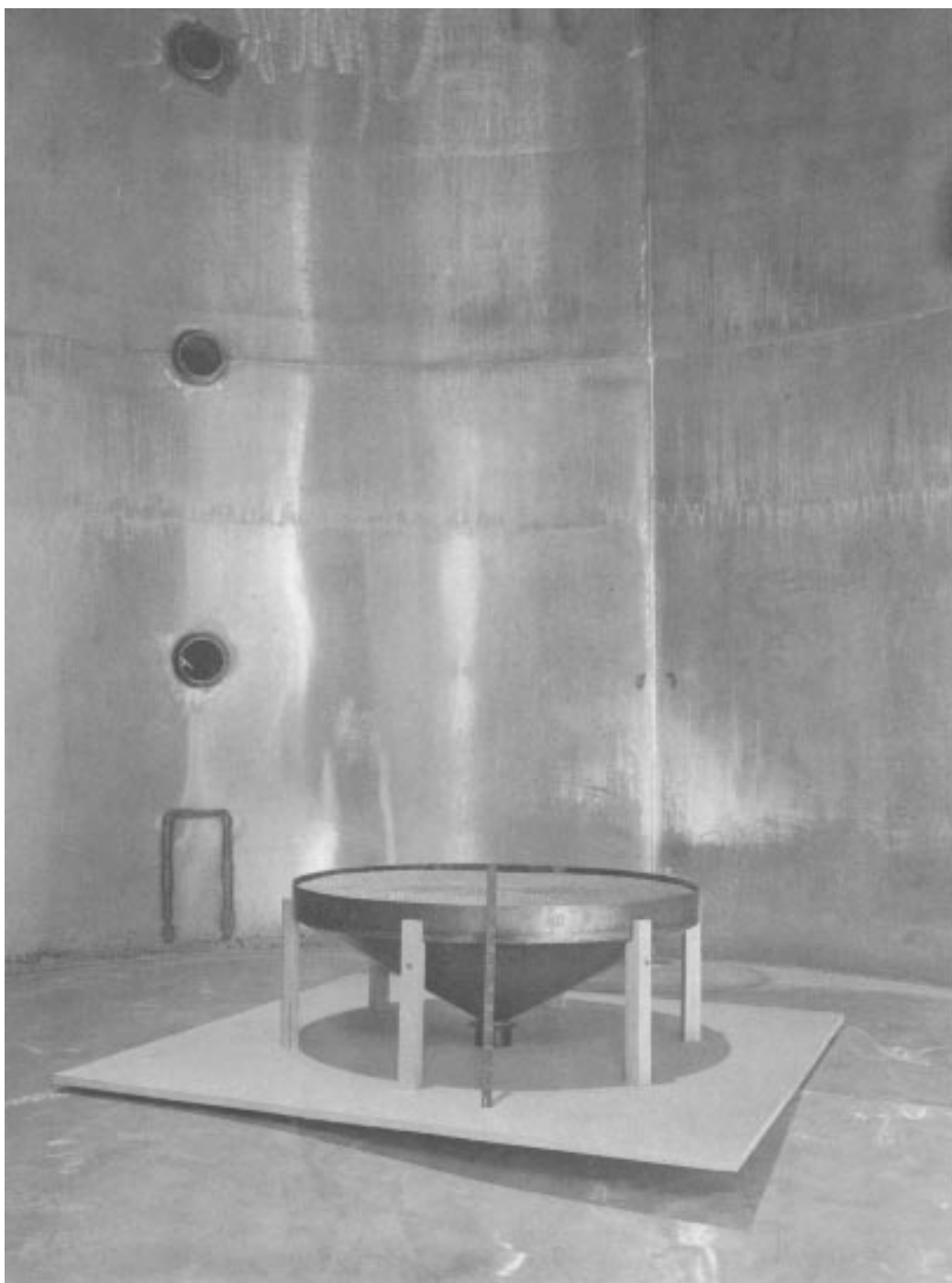
Figure A.42. Stainless Steel Screen and Support Used in Burning of Flammable Materials
