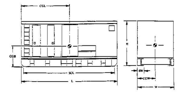
SCL - Skid Chamber Length L - Overall Length H- Overall Height CGW - Center of Gravity Width SW - Skid Width W - Overall Width CGL - Center of Gravity Length CGH - Center of Gravity Height
