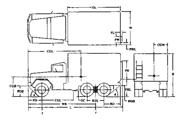
OL - Overall Length Body PW - Projection Width PH - Projection Height PL - Projection Length L - Overall Length CGW - Center of Gravity Width WB - Wheel Base FOH - Front Overhang Height ROH - Rear Overhang Height GCL - Ground Clearance Location a - Angle of Approach F - Front Axle Load W - Overall Width
