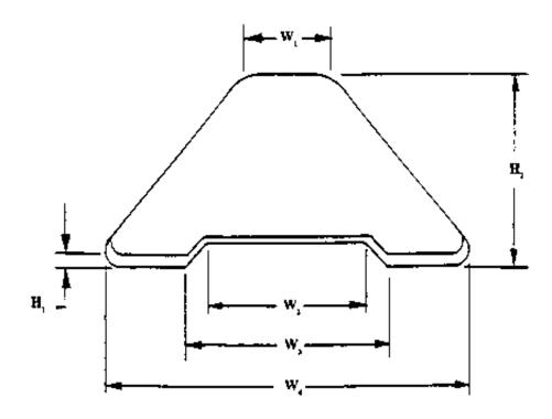
Figure 7 - Track Shoe Pad Dimensions (footprint data)
