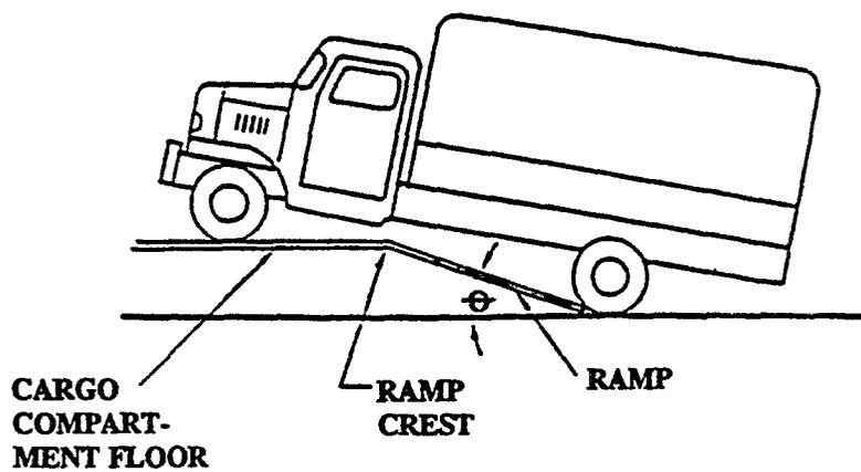
**FIGURE 3. Ramp crest angle**
