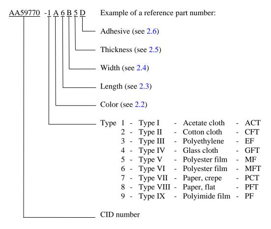
AA59770-1A6B5D identifies acetate cloth, black, 216 feet long, 0.250 inch wide, 0.0080 inch thick, rubber thermosetting adhesive.
