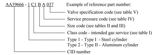
AA59666 - 1 C1 B A 037 indicates: steel cylinder; intended gas service 49456, butane; diameter 6.75 inches, height 21 inches, tare weight 20 pounds, water capacity 21.50 pounds, volume 596 cubic inches; service pressure 240 psig; valve type V22-660-13.
