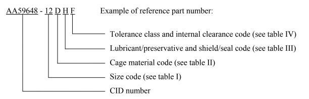
AA59648-12CHF indicates: 1.8750 bore diameter; 4.5000 outside diameter; 1.0625 width; machined non metallic (phenolic) cage; a double shield bearing lubricated in accordance with MIL-PRF-81322; ABEC-5 tolerance class, normal clearance.
