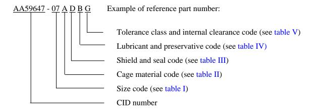
AA59647-07 A D B G indicates: 1.2500 bore diameter; 2.7500 outside diameter; 0.6875 width; corrosion resistant steel cage; a single seal bearing lubricated in accordance with MIL-PRF-81322; ABEC-3 tolerance class, loose internal clearance.
