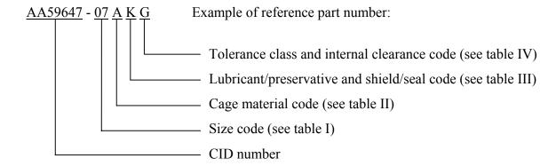
AA59647-07 A K G indicates: 1.2500 bore diameter; 2.7500 outside diameter; 0.6875 width; pressed steel or molded plastic cage; a single seal bearing lubricated in accordance with MIL-PRF-81322; ABEC-5 tolerance class, loose internal clearance.
