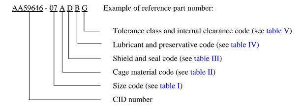
AA59646-07 A D B G indicates: 2.1250 bore diameter; 3.4375 outside diameter; 0.6250 width; corrosion resistant steel cage; a single seal bearing lubricated in accordance with MIL-PRF-81322; ABEC-3 tolerance class, loose internal clearance.
