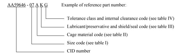
AA59646-07 A K G: indicates; 2.1250 bore diameter; 3.4375 outside diameter; 0.6250 width; pressed steel or molded plastic cage; a single seal bearing lubricated in accordance with MIL-PRF-81322; ABEC-5 tolerance class, loose internal clearance.
