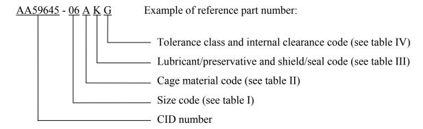
AA59645-06 A K G indicates: 1.1250 bore diameter; 2.1250 outer diameter; 0.5000 width; pressed steel or molded plastic cage; single seal bearing lubricated in accordance with MIL-PRF-81322; ABEC-5 tolerance loose internal clearance.
