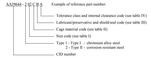
AA59644-2 02 C B A indicates: corrosion resistant steel; 0.1250 bore diameter; 0.5000 outer diameter; 0.1719 width; machined brass or bronze cage; open bearing; lubricant in accordance with MIL-PRF-81322; tolerance class ABEC-1, tight internal clearance.
