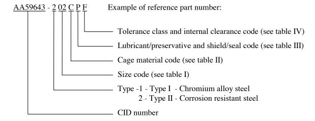
AA59643 - 2 02 C P F indicates: corrosion resistant steel; 0.0469 bore diameter; 0.1562 outer diameter; 0.0937 width; machined brass or bronze cage; single shield and single seal, lubricant in accordance with DOD-G-24508; ABEC-3P tolerance, normal internal clearance.
