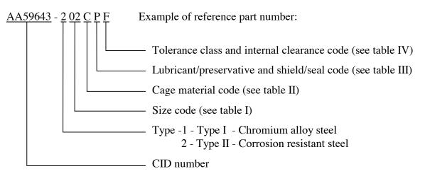
AA59643 - 2 02 C P F indicates: corrosion resistant steel; 0.0469 bore diameter; 0.1562 outer diameter; 0.0937 width; machined brass or bronze cage; single shield and single seal, lubricant in accordance with DOD-G-24508; ABEC-3P tolerance, normal internal clearance.
