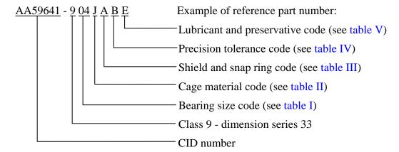
AA59641 - 9 04 J A B E indicates: boundary dimension series 33; bore diameter 20 mm, outside diameter 52 mm, width 22.2 mm; pressed steel cage; open (no shields); ABEC-1 tolerance class, normal radial internal clearance; filled with grease in accordance with DOD-G-24508.
