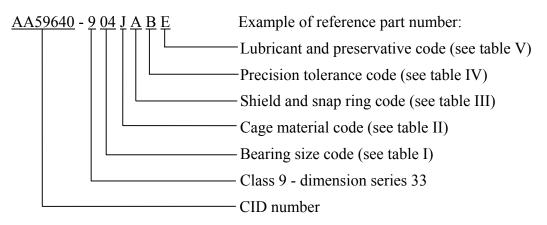
AA59641 - 9 04 J A B E indicates: boundary dimension series 33; bore diameter 20 mm, outside diameter 52 mm, width 22.2 mm; pressed steel cage; open (no shields); ABEC-1 tolerance class, normal radial internal clearance; filled with grease in accordance with DOD-G-24508.
