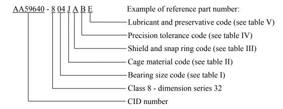
AA59640 - 8 04 J A B E indicates: boundary dimension series 32; bore diameter 20 mm, outside diameter 47 mm, width 20.6 mm; pressed steel cage; open (no shields); ABEC-1 tolerance class, normal radial internal clearance; filled with grease in accordance with DOD-G-24508.
