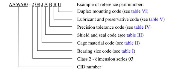
AA59630 - 2 08 J A B B U indicates: boundary dimension series 03; bore diameter 40 mm, outside diameter 90 mm, width 23 mm; pressed steel cage; open, no shield or seal; ABEC-1 tolerance class; filled with grease in accordance with MIL-PRF-81322; universal duplex mounting.
