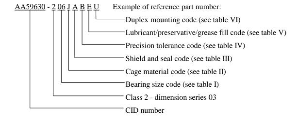
AA59630 - 2 06 J A B E U indicates: boundary dimension series 03; bore diameter 30 mm, outside diameter 72 mm, width 19 mm; pressed steel cage; open (no shields or seals); ABEC-1 tolerance class, normal radial internal clearance; filled 25% to 50% with grease in accordance with DOD-G-24508; universal duplex mounting.
