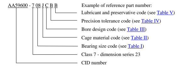
AA59600 - 7 08 J C B B indicates: boundary dimension series 23; bore diameter 40 mm, outside diameter 90 mm, width 33 mm; pressed steel cage; cylindrical bore (no shields or seals); ABEC-1 tolerance class, normal radial internal clearance; filled 25-50 percent with grease in accordance with MIL-PRF-81322.
