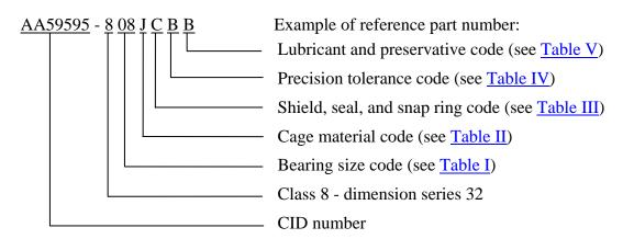
AA59595 - 8 08 J C B B indicates: boundary dimension series 32; bore diameter 40 mm, outside diameter 80 mm, width 30.2 mm; pressed steel cage; double contact seal with snap ring; ABEC-1 tolerance class, normal radial internal clearance; filled with grease in accordance with MIL-PRF-81322.
