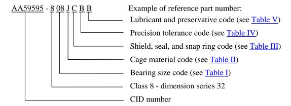
AA59595 - 8 08 J C B B indicates: boundary dimension series 32; bore diameter 40 mm, outside diameter 80 mm, width 30.2 mm; pressed steel cage; double contact seal with snap ring; ABEC-1 tolerance class, normal radial internal clearance; filled with grease in accordance with MIL-PRF-81322.
