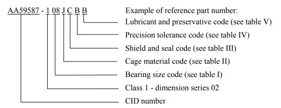
AA59587 - 1 08 J C B B indicates: boundary dimension series 02; bore diameter 40 mm, outside diameter 80 mm, width 18 mm; pressed steel cage; single shield on filling slot side; ABEC-1 tolerance class, normal radial internal clearance; filled with grease in accordance with MIL-PRF-81322.
