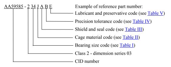
AA59585 - 2 34 J A B E indicates: boundary dimension series 03; bore diameter 170 mm, outside diameter 360 mm, width 72 mm; pressed steel cage; open; ABEC-1 tolerance class, normal radial internal clearance; filled with grease in accordance with DOD-G-24508.
