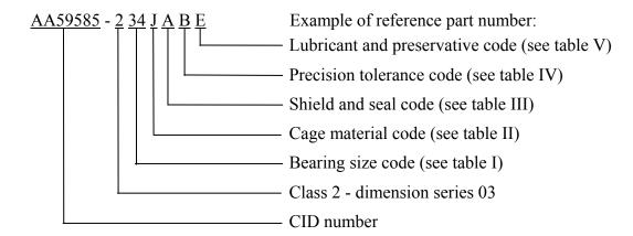
AA59585 - 2 34 J A B E indicates: boundary dimension series 03; bore diameter 170 mm, outside diameter 360 mm, width 72 mm; pressed steel cage; open; ABEC-1 tolerance class, normal radial internal clearance; filled with grease in accordance with DOD-G-24508.
