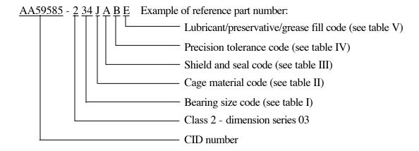
AA59585 - 2 34 J A B E indicates boundary dimension series 03; bore diameter 170 mm, outside diameter 360 mm, width 72 mm; pressed steel cage; open; ABEC-1 tolerance class, normal; filled 25-50% with grease in accordance with DOD-G-25508.
