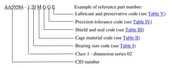
AA59584 - 1 20 M G G E indicates: boundary dimension series 02; bore diameter 100 mm, outside diameter 180 mm, width 34 mm; machined brass cage; open with snap ring; ABEC-3 tolerance class, greater than normal radial internal clearance; filled with grease in accordance with DOD-G-24508.
