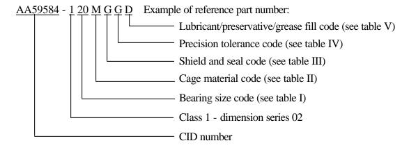
AA59584 - 1 20 M G G D indicates: boundary dimension series 02; bore diameter 100 mm, outside diameter 180 mm, width 34 mm; machined brass cage; open with snap ring; ABEC-3 tolerance class, greater than normal radial internal clearance; filled up to 25% with grease in accordance with DOD-G-24508.
