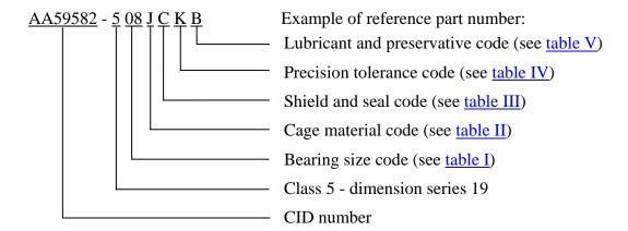
AA59582 - 5 08 J C K B indicates: boundary dimension series 19; bore diameter 40 mm, outside diameter 62 mm, width 12 mm; pressed steel cage; double shield; ABEC-5 tolerance class, normal radial internal clearance; filled with grease in accordance with MIL-PRF-81322.
