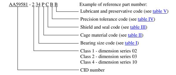
AA59581 - 2 34 P C B B indicates: boundary dimension series 03; bore diameter 4 mm, outside diameter 16 mm, width 5 mm; molded plastic cage; double shield; ABEC-1 tolerance class, normal radial internal clearance; filled with grease in accordance with MIL-PRF-81322.
