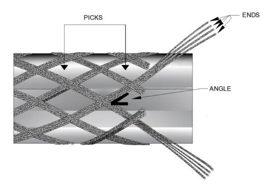
Angle. The smaller of the two angles formed by a shielding strand and the axis of the cable being shielded.
