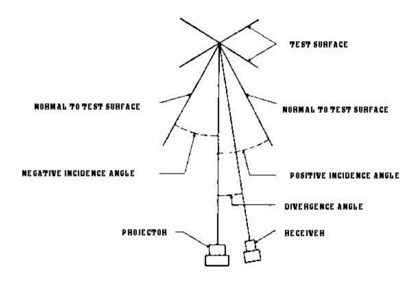
Figure I - Incidence and Divergence Angles
