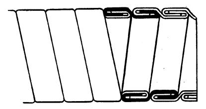
Figure 1. Type I Hose Construction
