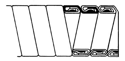
Figure 2. Type II Hose Construction
