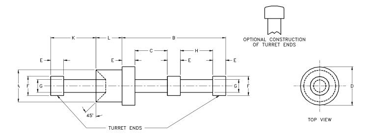
FIGURE 1. Single-double feedthru terminal stud.
