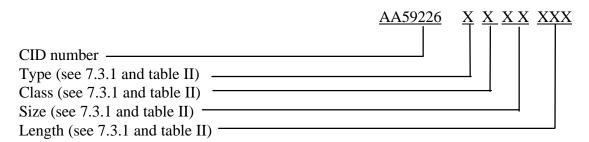
7.3.1 Type, class, and size. The type, class, and size of hoses (see 2.) are converted to a numeric code (see table II). The length is the number in feet of the hose. An example of the PIN is as follows:
