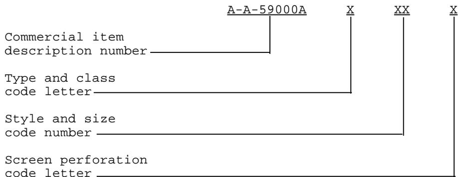
7.6.1 Type and class. The type and class of strainer (see 1.2) are identified by a single letter (see table V).
