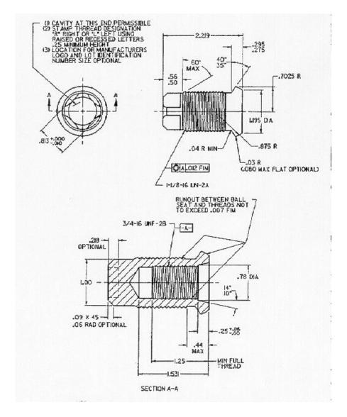
NOTE:1. Unless otherwise specified, tolerances are  $\pm$  .010 on decimal and  $\pm$ 1° on angular dimensions. Do not scale.
