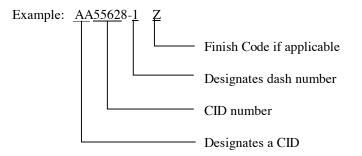
AA55628-1Z indicates Nut, plain, cap, high crown, .138-32 UNC-2B thread, carbon steel, Zinc plated.
