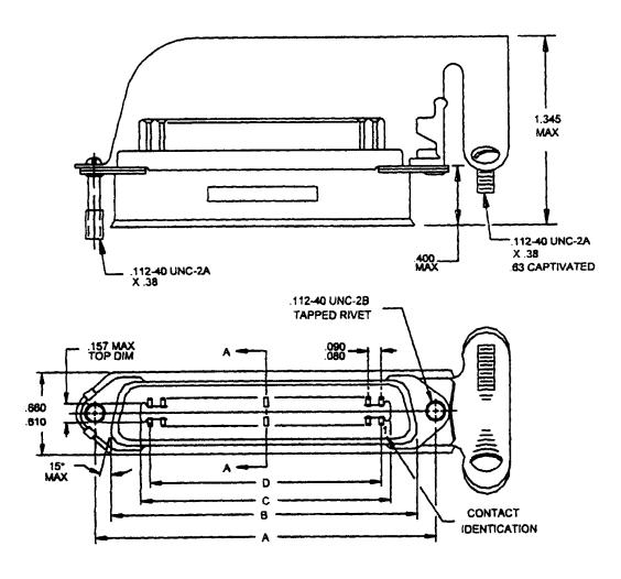
FIGURE 1. <u>Dimensions and configurations</u>.
