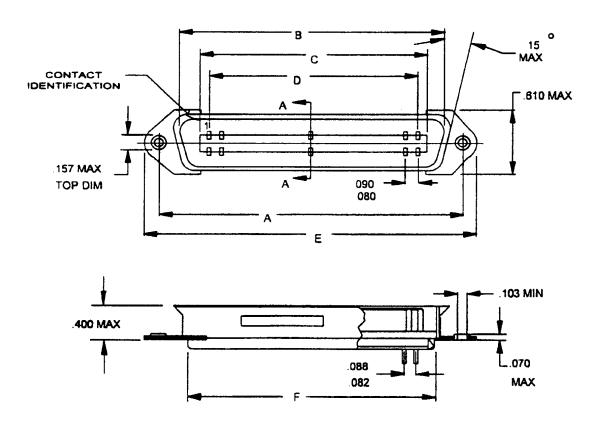
FIGURE 1. <u>Dimensions and configurations</u>.
