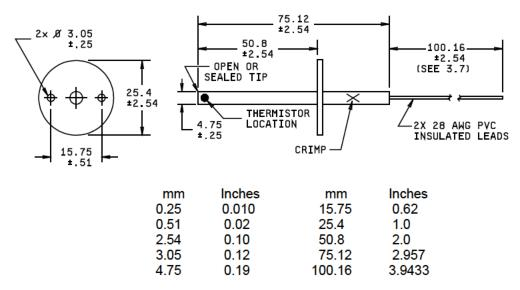
FIGURE 1. Resistor, thermally sensitive (thermistor probe).
