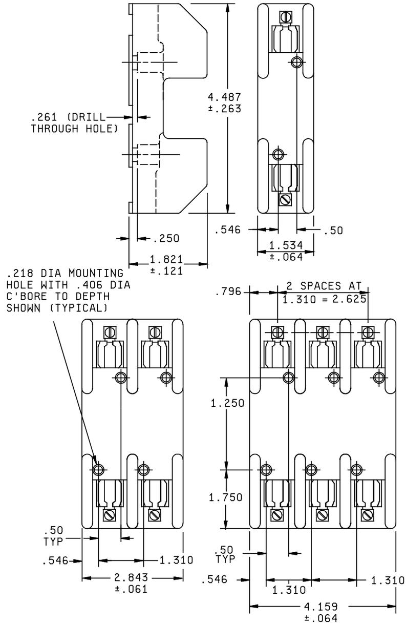
FIGURE 1. Configuration and dimensions.
