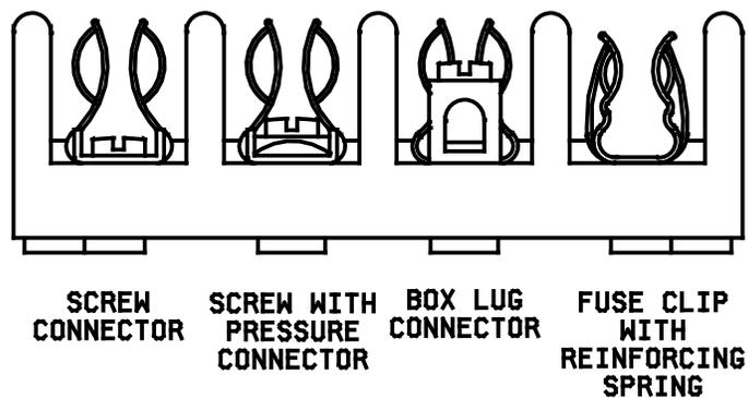
FIGURE 2. Wire termination configuration.
